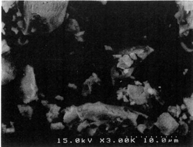
Fig. 4. Photograph of alumina ( $\text{Al}_2\text{O}_3$ ) grains taken with a scanning electron microscope. The total length of the calibration bar is  $10\ \mu\text{m}$  ( $1.0\ \mu\text{m}$  between tick marks). From pictures taken with a lower magnification we have determined that the average particle size is approximately  $8\ \mu\text{m}$ . Individual grains are tabular and have a fractured surface.
