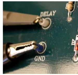
Probe tip, connected to terminals on circuit board. The alligator clip is connected to the GND terminal. Lay the tips on their sides, as shown here.
