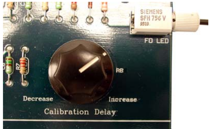
Figure II-3. Calibration delay. This knob on the circuit board adds a delay to the receiver signal so that you can position the receiver pulse at a convenient place on the scope display. Initially you should turn this knob to the 1-O’Clock position.
