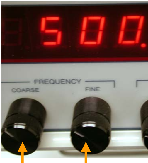
Figure III-2. Adjust the frequency to 500 kHz, using the COARSE and FINE knobs. Any value between 480 and 520 kHz is ok.
