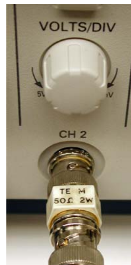
Figure III-4. Use a 50 Ohm terminator at the end of the BNC cables, where they are connected to the oscilloscope inputs. This avoids signal reflections at the high input impedance of the scope, yielding a cleaner waveform. (Your terminator may look different from the one shown here.)
