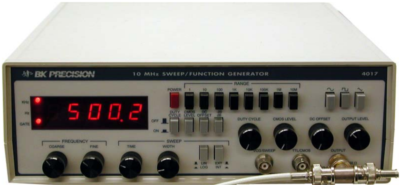
Figure III-1. Function Generator. You will set it up to produce a 500-kHz square wave. (Instead of the BNC tee, shown here on the output, you should use a splitter to divide the signal into two cables.)
