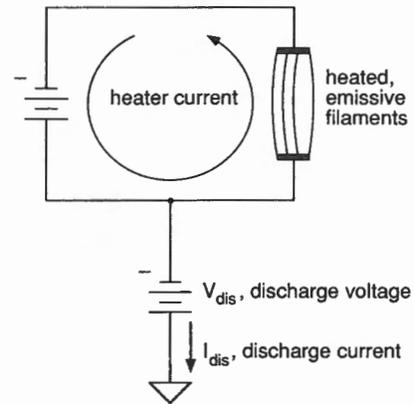
Fig. 2. Schematic of the filament circuit. The filaments are heated by the heater current and are biased negatively at a voltage  $V_{\text{dis}}$  to emit electrons. When a plasma is formed, a discharge current  $I_{\text{dis}}$  flows through the biasing power supply. The circuit shown here is completed by the vacuum vessel, which acts as a grounded anode that collects the current emitted by the filaments. When there is no plasma,  $I_{\text{dis}} = 0$ .
