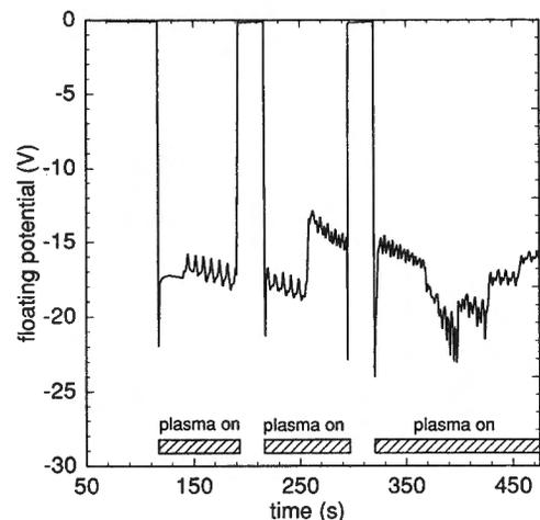
Fig. 7. Time history of the floating potential  $V_{\text{float}}$  of the test body. The floating potential is negative and is modulated at the rotation frequency. As the rate of shedding decreases, the floating potential becomes more negative.
