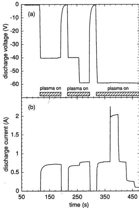
Fig. 5. Time histories of (a) discharge voltage  $V_{\text{dis}}$  and (b) discharge current  $I_{\text{dis}}$ . There is no plasma when  $I_{\text{dis}} = 0$ . The plasma was deliberately switched off and on to observe the plasma's effect on dust shedding. During the plasma-on intervals we operated at several different discharge voltages and currents.
