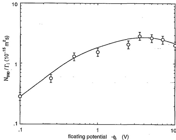
FIG. 3. Number of trapped ions  $N_{\text{trap}}$  per unit of incoming ion flux,  $\Gamma_i = n_i v_i$ . These results from Eq. (4) are valid if  $N_{\text{trap}} \ll Q_D/e$ . Unlike Fig. 2, these data are independent of  $\lambda_{\text{mfp}}$ .
