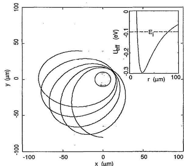
FIG. 1. Trapped hydrogen ion orbiting around a negatively charged dust grain. Parameters are  $E_i = -0.1$  eV,  $\phi_f = -2.5$  V, and others listed for Fig. 2.  $U_{\text{eff}}(r)$  is shown in the inset.
