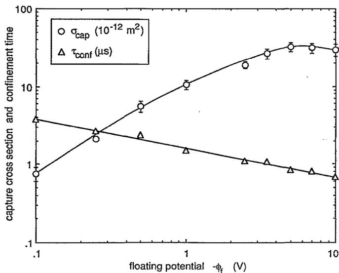
FIG. 2. Monte Carlo simulation results for captured hydrogen ions, born by charge exchange. The capture cross section  $\sigma_{\text{cap}}$  is computed from Eq. (2). Newly captured ions were followed until they were detrapped due to further collisions, yielding the confinement time  $\tau_{\text{conf}}$ . Parameters are  $a=10 \mu\text{m}$ ,  $\lambda_D=100 \mu\text{m}$ ,  $\lambda_{\text{mfp}}=3 \text{ mm}$ ,  $E_i=1 \text{ eV}$ . Error bars arise from counting statistics.
