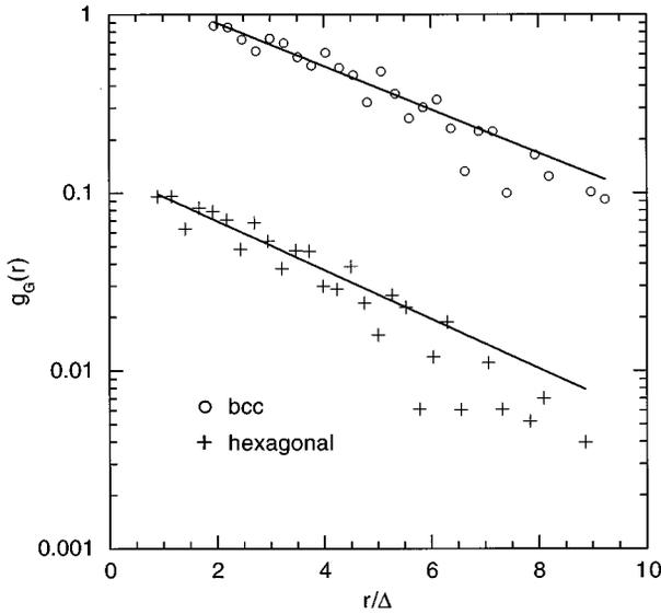
FIG. 3. The translational order-parameter correlation function  $g_G(r)$  for the bcc and simple-hexagonal crystals of Fig. 1, calculated in each horizontal plane and averaged over planes. The curves are fits by decaying exponentials which yield correlation lengths (in units of particle separation  $\Delta$ )  $\xi/\Delta=3.6\pm 0.2$  for bcc and  $\xi/\Delta=3.0\pm 0.2$  for hexagonal.
