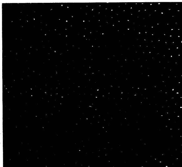
FIG. 2. Image of the particle cloud in a plane above the lower electrode. The area shown is 7.7 \times 7.7 \text{ mm}^2 and contains 724 particles of 7- \mu\text{m} diameter.
