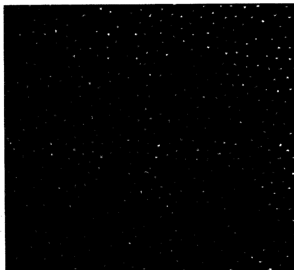
FIG. 2. Image of the particle cloud in a plane above the lower electrode. The area shown is 7.7 \times 7.7 \text{ mm}^2 and contains 724 particles of 7\text{-}\mu\text{m} diameter.
