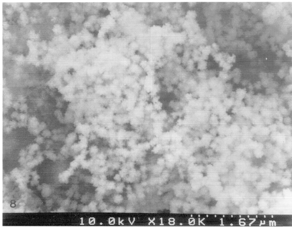
Fig. 7. Carbon grains collected after 420 min. The spheroids have a cauliflower-like surface structure. Particles of 1 \mu\text{m} size have stuck together, forming a coagulated string. The flatness of the spheroids indicates further growth by accretion following coagulation.
