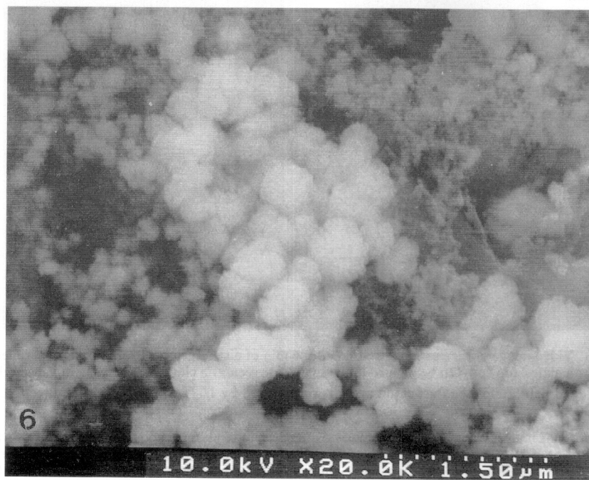
Fig. 5. Carbon grain collected after 20 min. Note the particles that appear to have stuck together.
