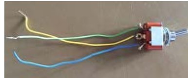
SPDT switch has 3 terminals
