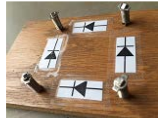
Board for rectifier
