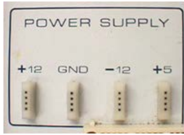
Figure 4-5. Power supply on prototyping board (left). Connect these using wires to the strips sketched on the right for convenient use. Note: some boards have only one strip per side, not two as shown here.
